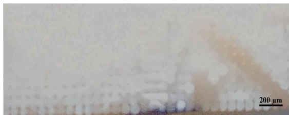
Fig. 4 - Gaps between layers before annealing.
