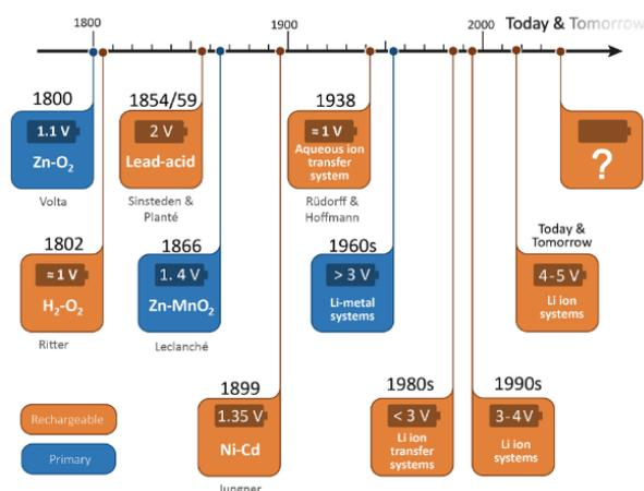
**Fig. 1** – The development of batteries from 1800 until today [9]
