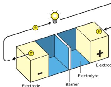
Fig. 3 – Working Principle of a Li-ion cell [1]
