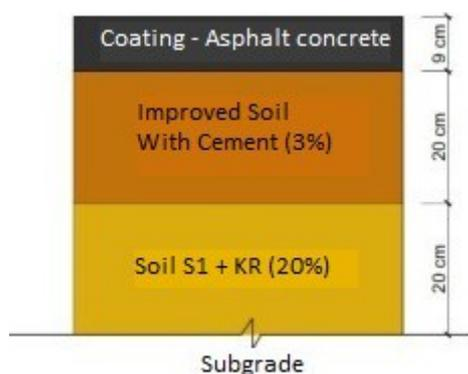
Fig. 2 - Paving Solution for Lane 1 [5].
