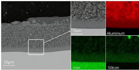
**Fig. 2** – SEM and EDS images of soldered aluminum on AISI H13 surface after 10 minutes of corrosion in molten aluminum (A383) at 720 °C.
